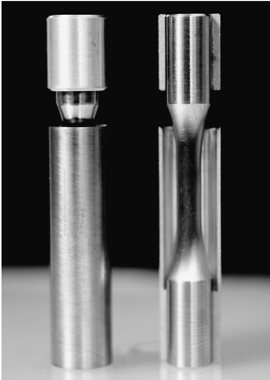
Fig. 2. Fatigue specimen with bushing and vial for containment of mercury.
